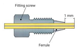
Figure 2. Schematic of the capillary connection.
