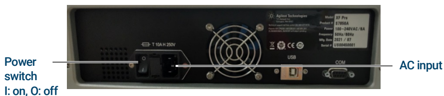
Figure 5 XF Pro rear panel - AC input and power switch.
