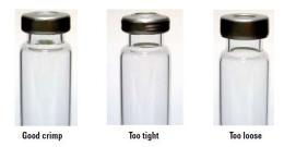
Use the same type and size of vials, caps, and seals for the purpose of setting the crimp tightness as you will for production crimping.
