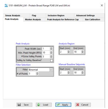
Figure 27 Peak Analysis tab in Global Configuration dialog
