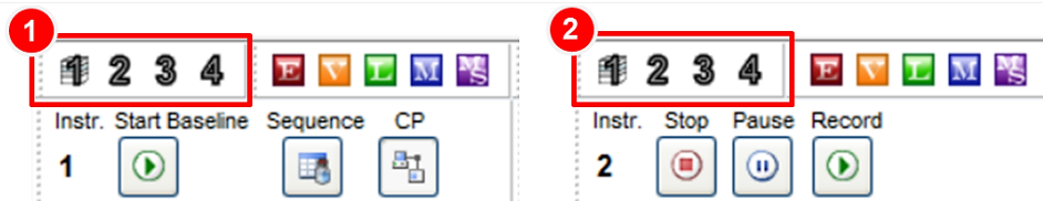
Figure 39 (1) Toolbar Instruments (red area) and Toolwindow Start/Stop for the controlled Instrument 1 and (2) Toolbar Instruments (red area) and Toolwindow Start/Stop for the not controlled Instrument 2
