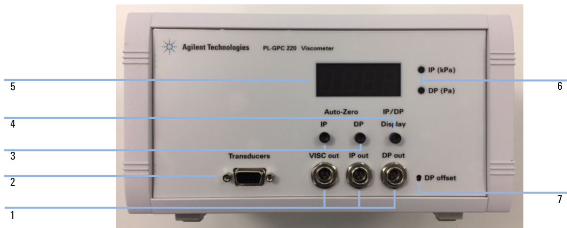
Figure 4 Front View of the Electronic Control Module for the Agilent GPC220 Viscometer
