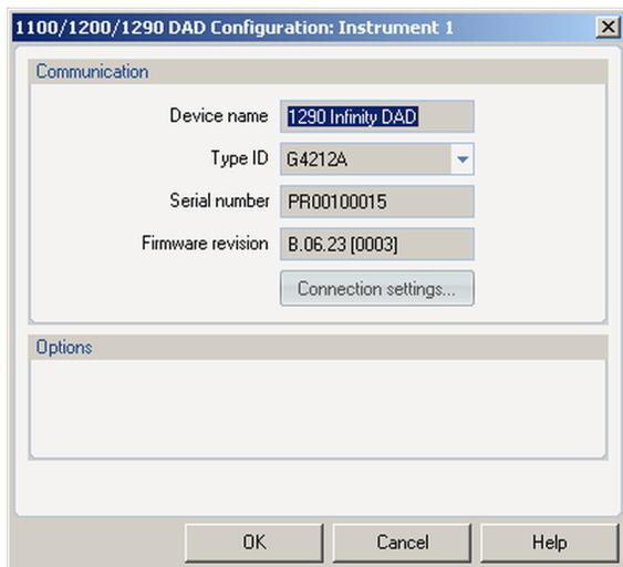
The screenshot shows a dialog box titled "1100/1200/1290 DAD Configuration: Instrument 1". It has a "Communication" section with the following fields: "Device name" (1290 Infinity DAD), "Type ID" (G4212A), "Serial number" (PR00100015), and "Firmware revision" (B.06.23 [0003]). There is a "Connection settings..." button below these fields. Below the "Communication" section is an "Options" section, which is currently empty. At the bottom, there are three buttons: "OK", "Cancel", and "Help".
