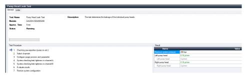
Figure 246 Pump Head Leak Test for the 2D-LC 1290 binary pump
