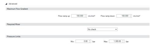
Figure 118 Advanced <sup>2</sup>D pump settings
