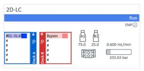
Figure 81 Heart Cut sampling/parking indicated by blue beam moving along, cut number and time in minutes
