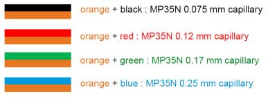
Figure 265 Color code for biocompatible capillaries
