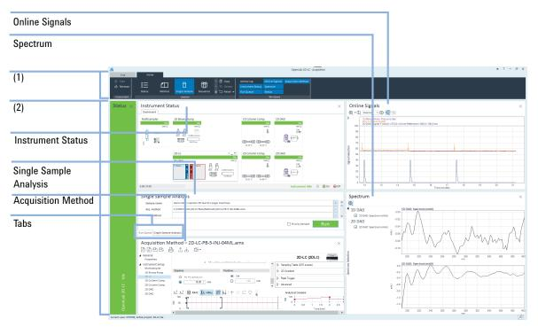
Figure 72 Overview of windows in Agilent Acquisition OpenLab CDS
