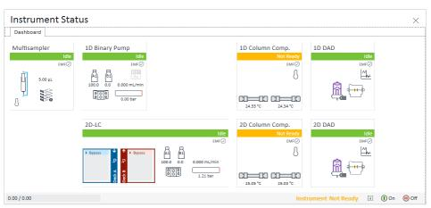
Figure 74 Instrument Status for a full 2D-LC Solution with UV detection
