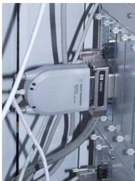
Figure 7 USB-GPIB Interface Connection
