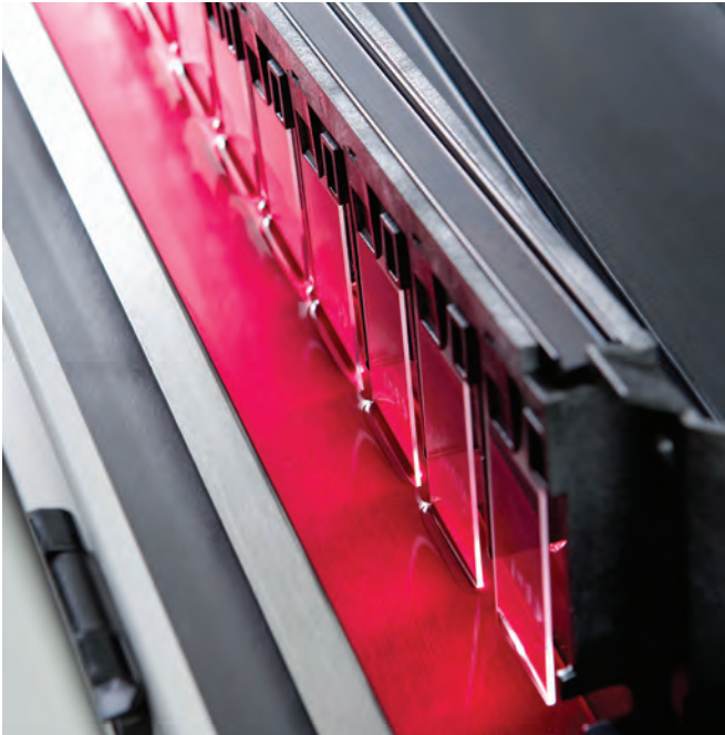
Figure 3.2 PT Link is a water bath method for antigen retrieval
