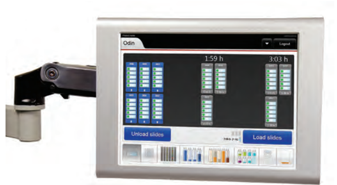
Figure 9.8 The scheduler software organizes the sequence of all individual steps an instrument must perform from start to end of the staining process for the given load of slides. For some instruments, the scheduler also calculates when slides will be completed.
