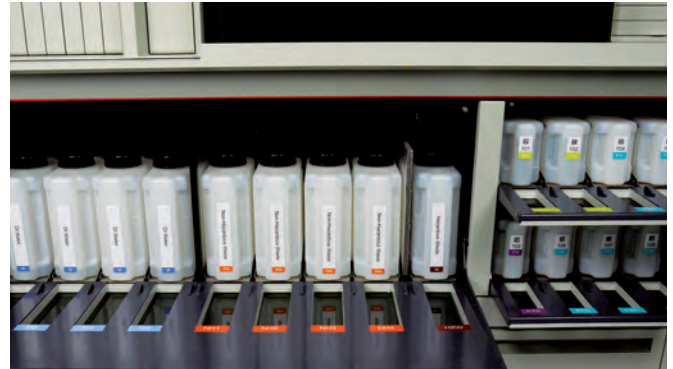
Figure 9.10 More onboard capacity for reagents and bulk fluid bottles can reduce hands-on time due to little or no reagent handling during the day.
