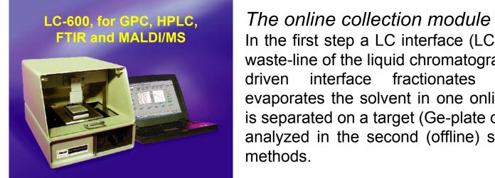
In the first step a LC interface (LC-600) is added to the waste-line of the liquid chromatography system. This PC driven interface fractionates the samples and evaporates the solvent in one online step. The mixture is separated on a target (Ge-plate or MALDI) and can be analyzed in the second (offline) step by spectroscopic methods.
