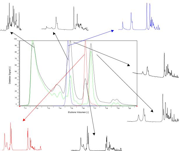
This second example shows a typical analytical question. A lacquer could not be fixed accurately on a polymer surface. The GPC analysis of good/bad samples showed, that the polymer was identical, but in the low molecular separation region one peak was more intensive for the "bad case". A direct FTIR coupling gave the solution for the problem: a slip agent was not removed from the surface in the "bad case".
