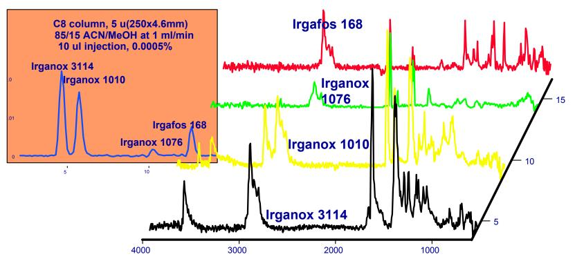
This "simulated" polymer (additives were added into the polymer, it is not a technical product) shows, that it is not necessary to get a baseline separation of each peak. The resulting spectra are "pure" enough to identify the additives using a library search.
