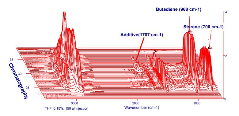
3. example: GPC-FTIR coupling after extraction
