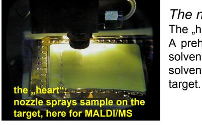
The nozzle The "heart" of this technique is the nozzle: A preheated gas stream ( $N_2$ , dry air) is mixed with the solvent/sample. When the spray leaves the nozzle, the solvent evaporates and the sample is deposited on the
