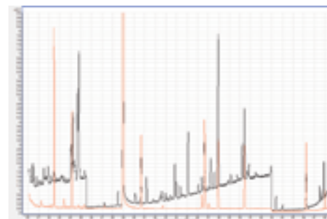
TIC of Mussel tissue extract (Black) overlaid with PCB Calibration Standard (Red) (1.5 µg/kg level).
