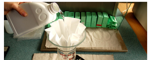
Figure 4A. Filtering the reagents after five days of usage.
