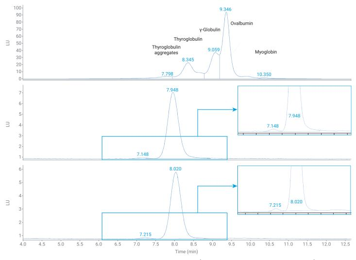
Figure 2. SEC chromatograms for AAV-9 and AAV-2, with an Agilent AdvanceBio SEC 300 Å standard column, using an Agilent Bio SEC-5 1000 Å column.
