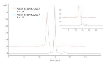
**Figure 3.** SEC chromatograms for a VLP using 1000 and 2000 Å Agilent Bio SEC-5 columns. The 2000 Å columns gave better resolution between the monomer and aggregate.
