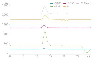
A low-dispersion setup and a 10 µL cell for light scattering detection result in excellent peak shapes for all signals.
