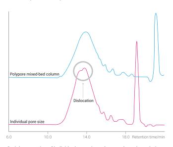
Serial connection of individual pore size columns, shear degradation, and adsorption to packing material can cause peak dislocations, peak tailing, and inaccurate results varying by as much as 10–20% from the true value. InfinityLab PlusPore columns can eliminate these issues.
