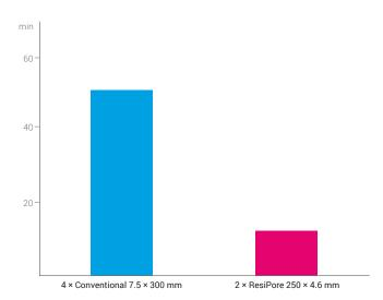
Flow rates can be increased for higher sample throughput. Using shorter, smaller internal diameter InfinityLab GPC/SEC columns with the 1290 Infinity II GPC/SEC System can reduce run times by up to 70%.
