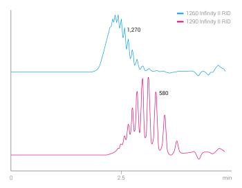
Used at microscale, the 1290 Infinity II RID has a low-volume detector cell and a reduced system delay volume relative to the 1260 Infinity II RID. This ultralow dispersion gives improved resolution, with the advantages of shorter run times and increased sample throughput.
