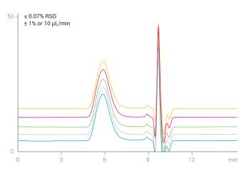
An accurate flow rate enables reproducible results. The value quoted has been calculated from analyses performed in THF at 40  $^{\circ}$ C.
