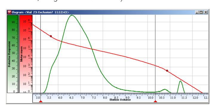
**Figure 2.** Selecting too low of an upper molar mass separation limit can yield artificial shoulders in chromatograms.
