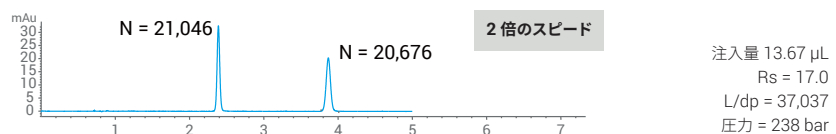
InfinityLab Poroshell 120 EC-C18, 4.6 x 100 mm (L1), 2.7 \mu m
