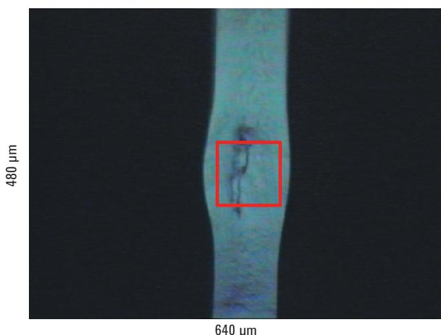
**Figure 1.** Visible image of the polymer cross-section with the defect of interest clearly visible in the center. The red box shows the location and area of the micro-ATR analysis.
