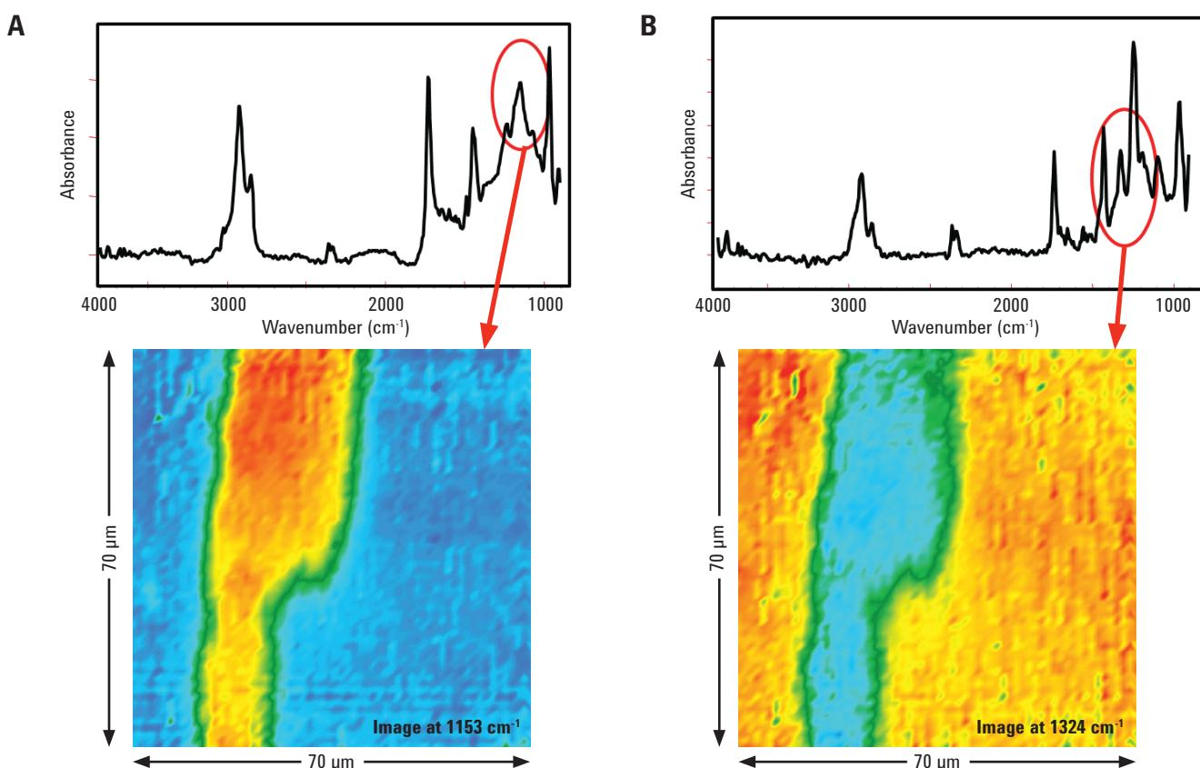
**Figure 3.** Chemical images and spectra from the measured sample. 3A. A chemical image where warm colors highlight areas of high absorbance intensities associated with what Resolutions Pro identified as an acryloid compound. 3B. A chemical image showing regions where intrinsic absorbances associated with the bulk polymer are present (warm colors) or absent (cool colors).
