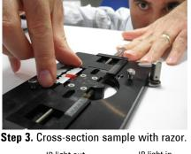
This mode provides for direct and real-time monitoring of the quality of contact (i.e., has the sample made complete contact across the entire field of view), which allows for extremely low levels of pressure to be applied. And it is this extremely low level of pressure that now allows for delicate and thin samples to be mounted, cross-sectioned end on, without any need for sample support using resin.
