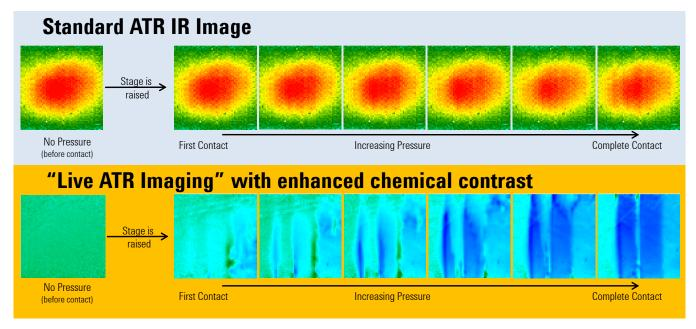
Figure 3. Comparison of a standard ATR IR image and Agilent's "Live ATR imaging" with enhanced chemical contrast—clearly showing the latter can detect first contact of the ATR crystal with the sample and that contact quality can be monitored real-time as the pressure is increased and before any data collection
