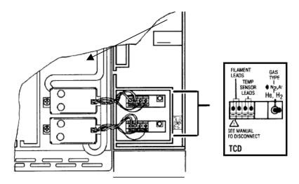
Special care should be taken when disconnecting the TCD filament leads, which run from the detector to the detector interface card. Use a small blade screwdriver to push down on the connector tabs while pulling out the wires.
