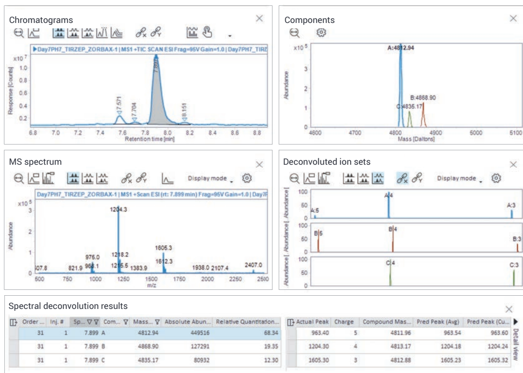
Figure 2. Data review for tirzepatide after seven days of storage at 5 °C and pH 7. The total ion chromatogram shows peaks corresponding to tirzepatide and its related impurity products. The mass spectrum at 7.89 minutes confirms the elution of tirzepatide, with the presence of +3, +4, and +5 charge states.
