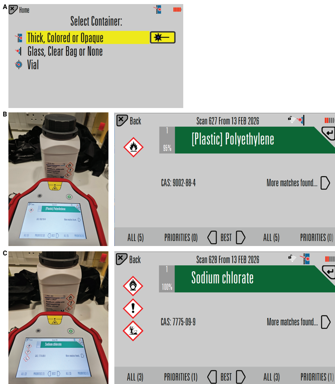
Figure 4. (A) The Agilent Resolve Tactical analyzer performs three types of measurements: through-barrier (thick, colored, or opaque), surface (glass, clear bag, or none), and vial mode. Using surface mode (B), the onboard algorithm matched the scan of the container to polyethylene. In SORS through-barrier mode (C), the Resolve detected the contents of the container and displayed the relevant hazards. This information enables appropriate measures to be taken before plastic disposal.
