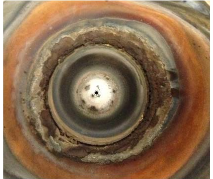
Bad Dirty sampling cone whose orifice is nearly clogged.
