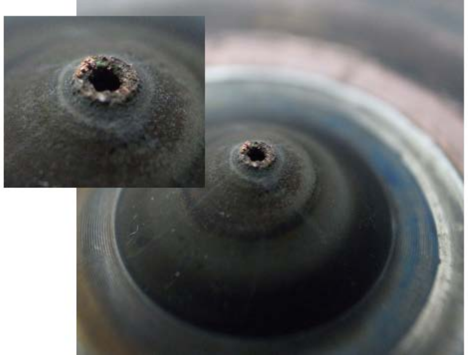
Bad Sampling cone with distorted orifice.
