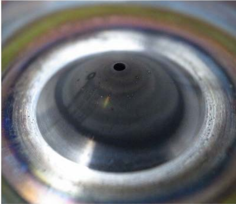
Good Sampling cone in good condition.
