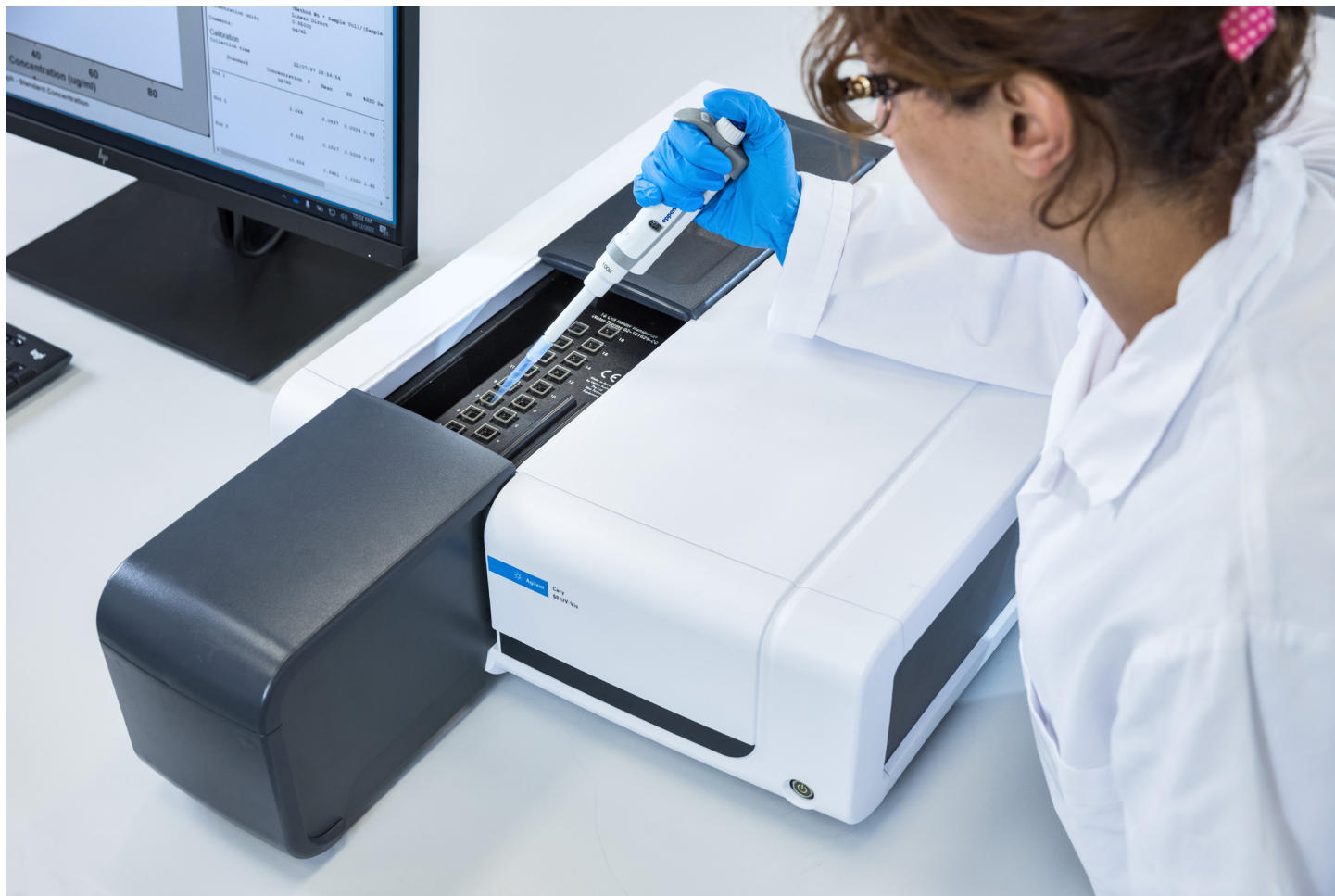
Figure 10. The Agilent Cary 60 UV-Vis with the 18-cell changer streamlines instrument qualification and enhances efficiency.
