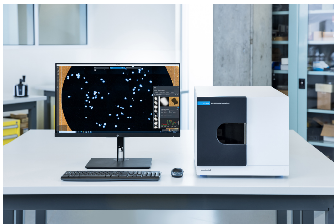
Figure 1. The Agilent 8700 LDIR chemical imaging system allows high-speed routine analysis of microplastics in drinking water, including the number of particles present in the sample, and their size and chemical composition.
