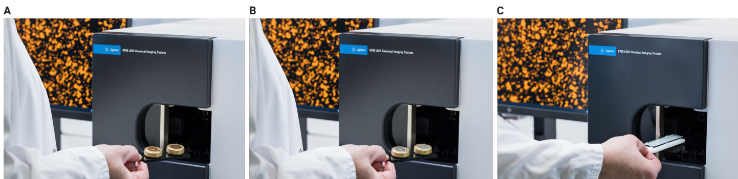
Figure 2. (A) Gold- and (B) aluminum-coated filters on holders, (C) low-e IR reflective slide. Samples can be prepared on either substrate, ready for direct analysis using an Agilent 8700 LDIR chemical imaging system.
