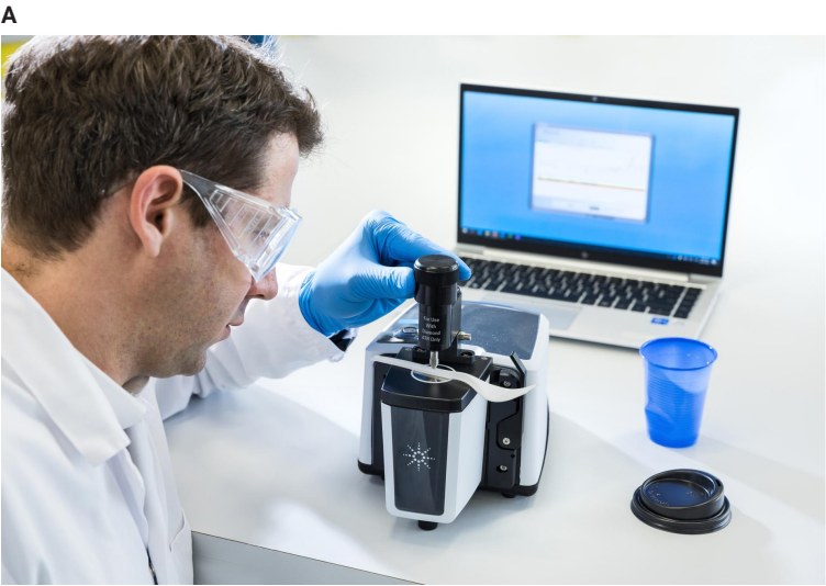
Figure 6. (A) Agilent Cary 630 FTIR spectrometer coupled with a diamond ATR module. (B) Example of Cary 630 FTIR qualitative analysis spectral data of plastic debris (red traces) and library hits (blue traces). The table shows the hit quality, library used, and the hit name for each sample. Color-coding the results based on the HQI score can be used to define confidence levels, helping users to interpret the results and reducing oversights that may lead to errors.
