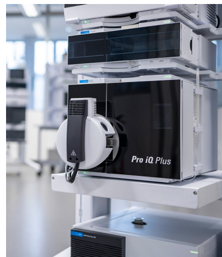
Figure 3. Agilent InfinityLab Pro iQ Plus instrument stacked with LC system on InfinityLab Flex Bench MS.
