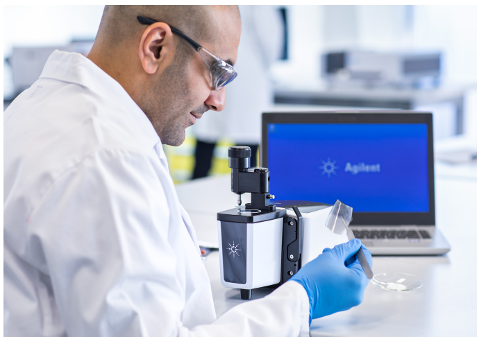
Figure 3. Analysis of a sheet-material using an Agilent Cary 630 FTIR with ATR sampling module.
