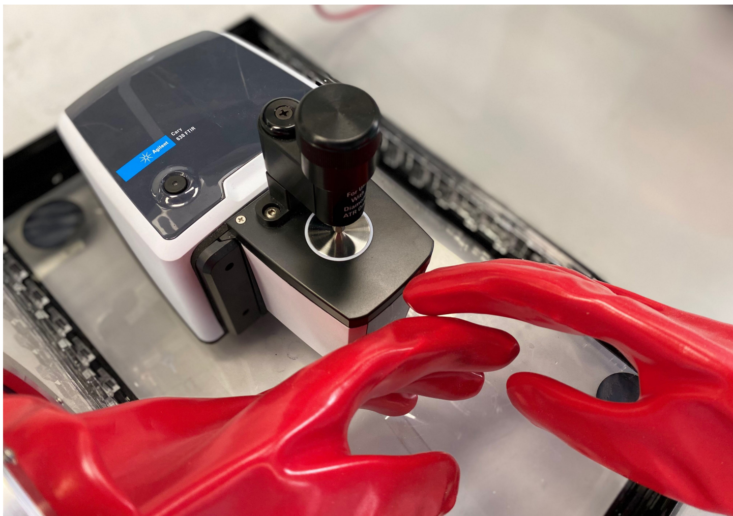
Figure 4. Agilent Cary 630 FTIR spectrometer inside a glovebox in which the moisture or oxygen level can be controlled. An ideal setup for LIB research applications.
