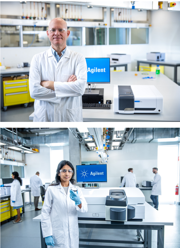
Figure 1. Agilent UV-Vis spectrophotometers used for color measurements include the Agilent Cary 60 UV-Vis spectrophotometer (top) and Agilent Cary 5000 UV-Vis-NIR spectrophotometer with an external diffuse reflectance accessory (DRA) (bottom).
