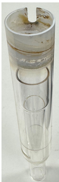
Figure 1. Devitrification of a quartz outer tube-set after 24 hours analyzing 1.5% TDS solution of Li, Na, Cs in 5% HNO 3 .
