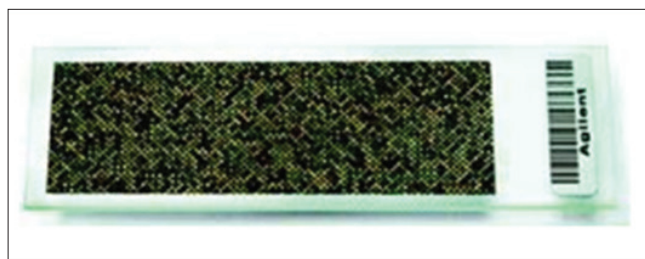
Figure 2. Agilent aCGH DNA microarray is a very high density microarray for oligonucleotide array-based CGH.
