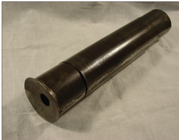
Figure 3. The Janssen microscope. The central tube allows for extension moving the objective away from the eyepiece allowing for magnification of between 3x – 10x.
