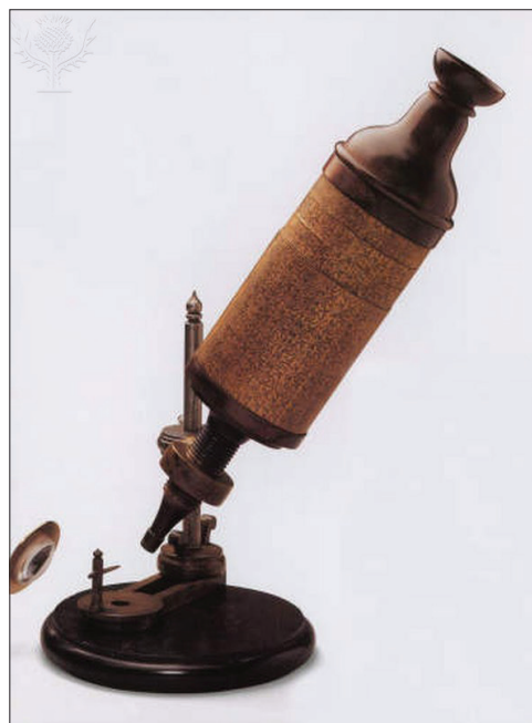
Figure 5. A replica of Hooke's compound microscope: notice the thread near the base which allowed for focusing.
