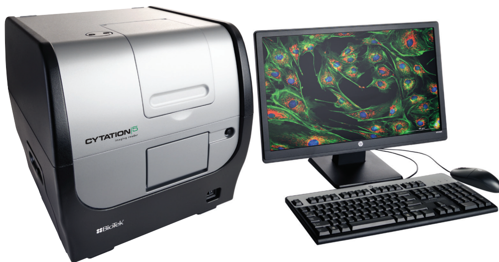
Figure 13. Cytation 5 Cell Imaging Multi-Mode Reader. This digital microscope provides wide field fluorescence and brightfield, color brightfield for histology applications (H&E staining) and phase contrast for imaging of cells without staining or fluorescent probes.
