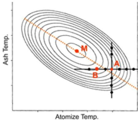
**Figure 2.** Using the ‘one variable at a time’ method of optimizing the graphite furnace temperature program often results in the analyst determining optimum temperatures (A & B in this diagram) that are some way off the true optimum (M in this diagram).
