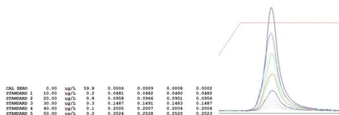
**Figure 8.** Determination of Al in water using the surface response method shows %RSD below 1% for all standards. The graph on the right is an overlay of the absorbance plots of three replicates of each of the five standards.
