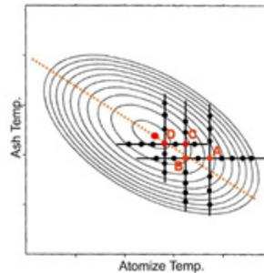
**Figure 3.** Through an iterative process, the analyst can optimize the ashing and atomization temperatures to get them closer to the optimum, but this is very time consuming.
