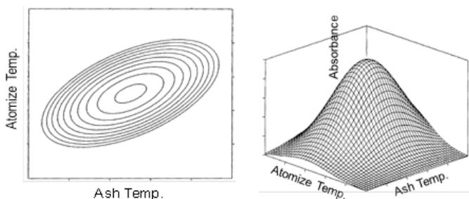
**Figure 4.** Surface response methodology can be used to determine the ashing and atomization temperatures that yield the best analyte absorbance. The figure on the left includes iso-response lines on a 2 dimensional surface. The 3 dimensional figure on the right includes a Z-axis of absorbance.
