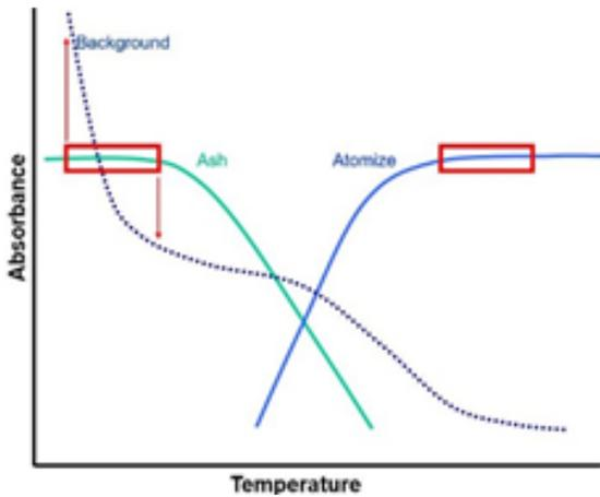
**Figure 1.** Using the “One variable at a time” optimization method requires the analyst to run many tests to determine the ashing and atomization temperatures that correspond to the highest analyte absorbance with the lowest background signal (the red rectangles).
