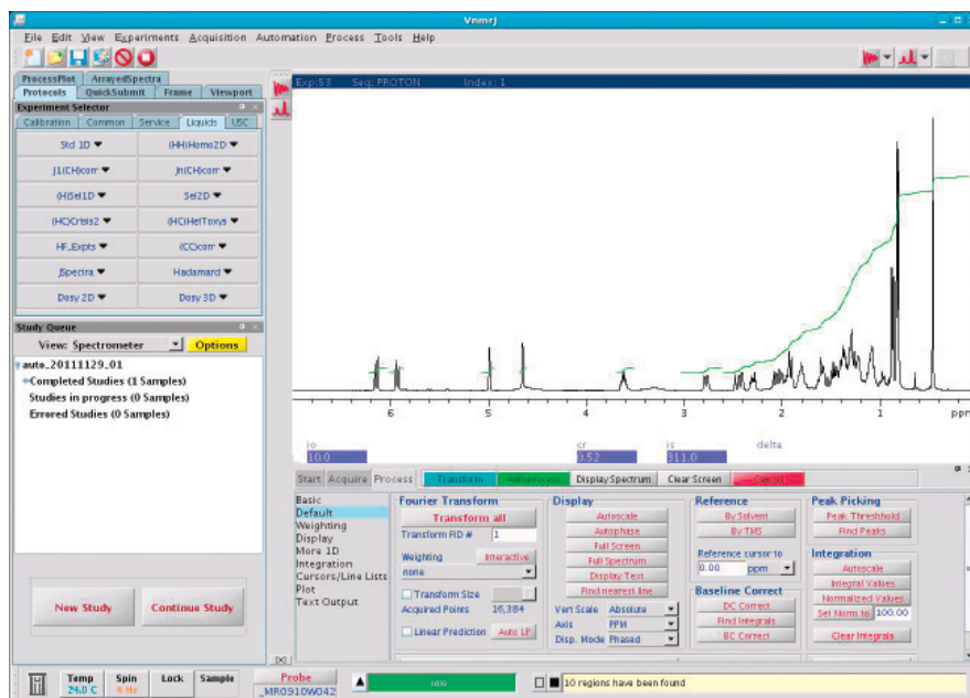
Figure 1. The StudyQ provides an intuitive interface for queuing sample acquisition. A variety of 1-D and 2-D experiments can be selected by clicking on the name in the top left panel. The experiment then drops into the queue (bottom left). Experiments can be reprioritized within the queue.
