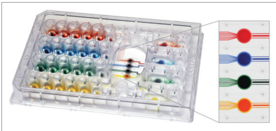
Figure 13. Representation of perfusion in a microfluidic 3D culture system. Cells are maintained in a predefined compartment by micropillars, allowing interplay with perfused media (Image courtesy of EMD Millipore Corporation).
