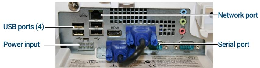
Figure 3. Controller ports (underside)
