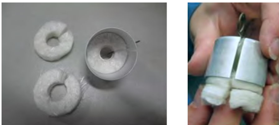
Figure 32 Insert insulation pieces into the nutwarmer cup
