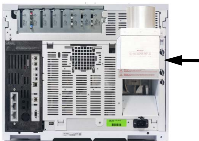
Figure 5. Exhaust deflector G3450-81650
