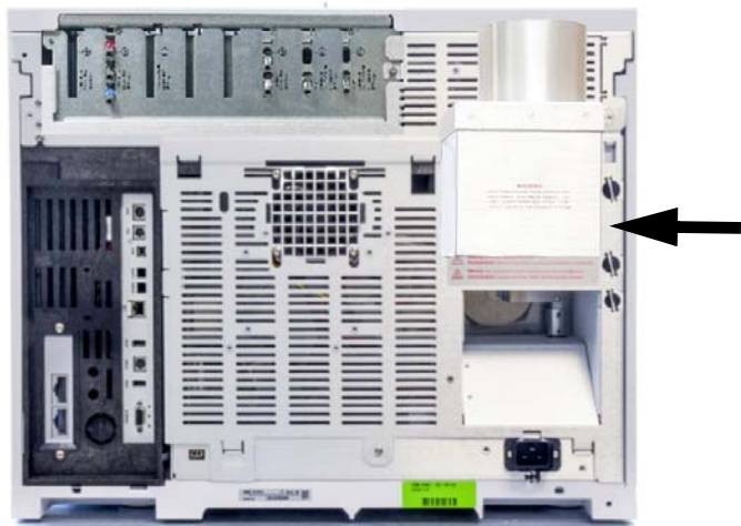
Figure 5. Exhaust deflector G3450-81650
