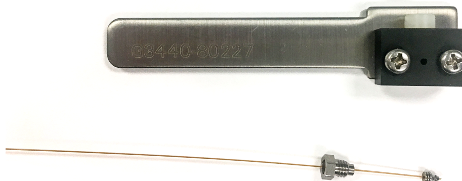
Figure 9. Thread the column through the internal nut, ferrule, and swaging tool
