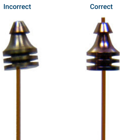
Figure 20. Incorrect and correct swaging symmetry
