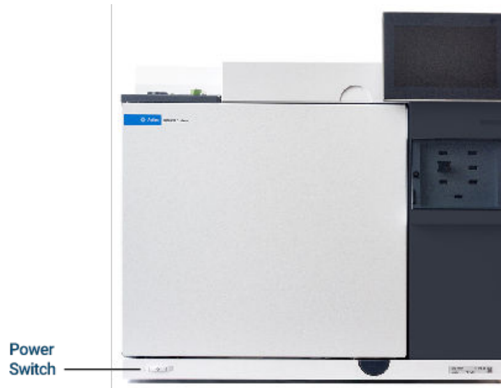
Figure 6. Power Switch location
