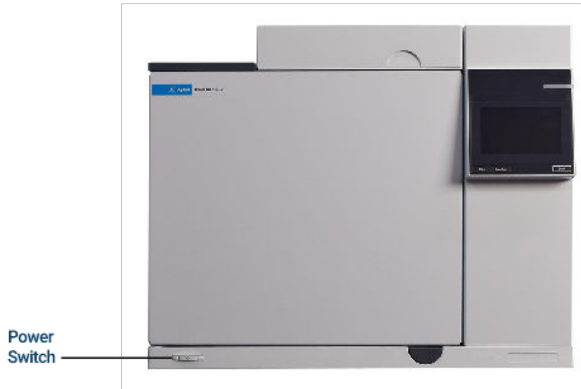
Figure 6. Power Switch location
