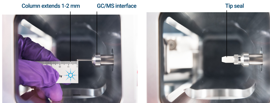
Figure 20. Installing a capillary column in the GC/MS interface for an EI XTR or a CI source
