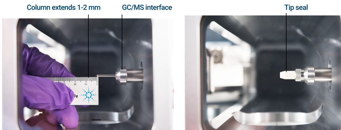
Figure 4. Installing a capillary column in the GC/MS interface for an EI XTR or a CI source
