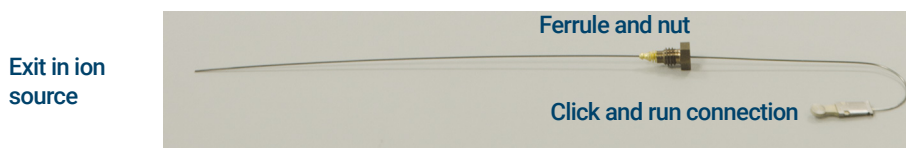
Figure 15. 9000 GC/MS Tail removed from GC/MS Interface
