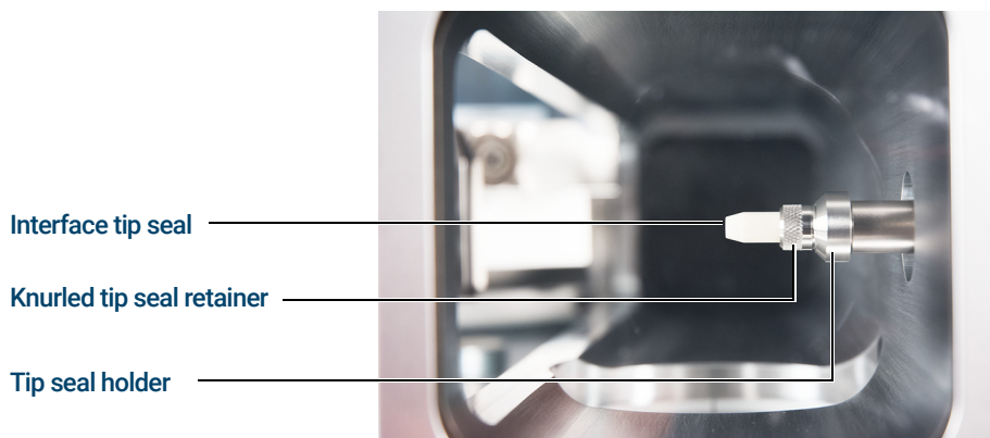
Figure 7. GC/MS interface tip seal
