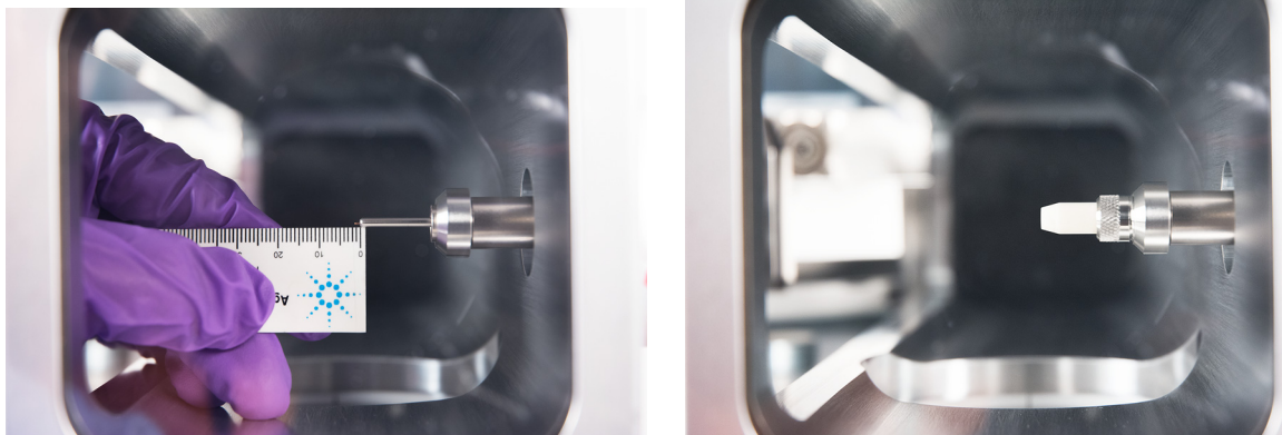
Figure 5. Installing a capillary column in the GC/MSD interface for an EI EXT, SS, Inert, or CI source.
