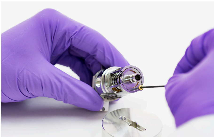
Figure 51 Secure the lens screw and lock ring insulator
