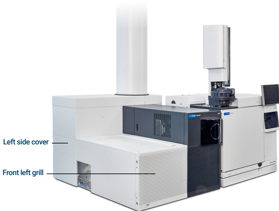
Figure 12. Remove covers to access the left side lifting handles
