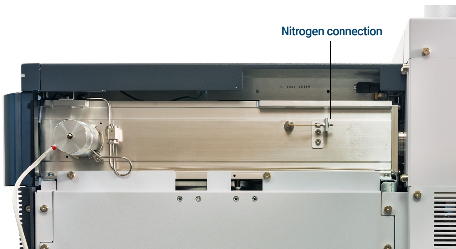
Figure 8. Collision cell nitrogen gas connection
