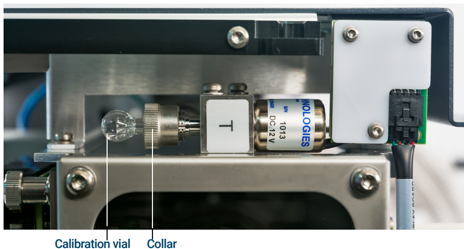
Figure 7. Removing the EI calibration vial
