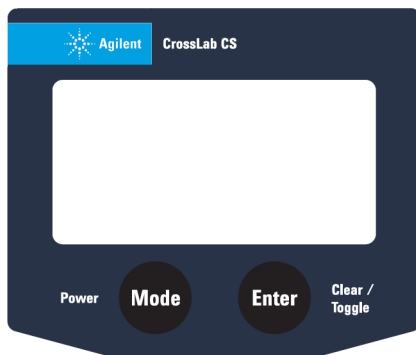
Figure 1. The Agilent CrossLab CS ADM flow meter front screen buttons.
