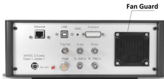
Figure 8. The fan guard on the back panel of the ExD Controller.
