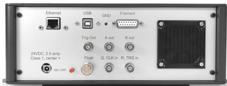
Figure 5. The ExD Controller back panel.
