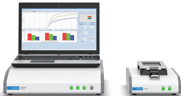
Figure 1. Agilent xCELLigence RTCA SP instrument. This consists of the plate station (housed inside a tissue culture incubator), analyzer, and laptop control unit (both housed outside the incubator).
