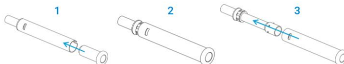
Figure 11 Illustrated view showing the disassembly of the ceramic outer tube-set
