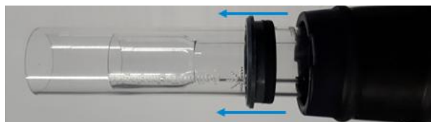
Figure 8 If the top seal is dislodged with the outer tube-set, slide the seal away from the torch body to remove
