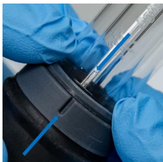
Figure 9 Align the torch body groove with the "T" mark on the outer tube-set
