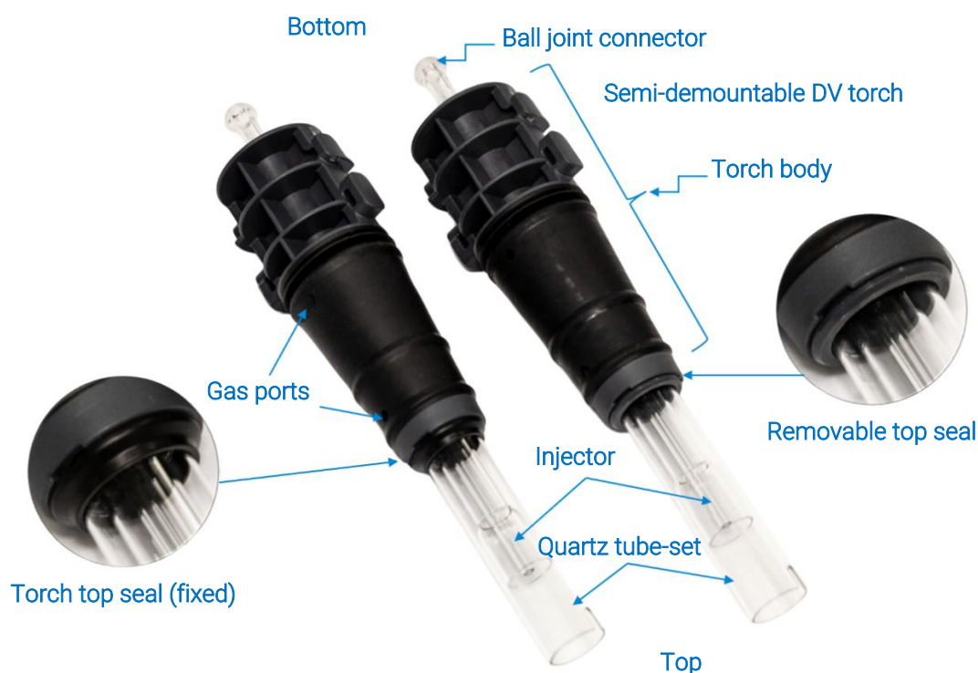
Figure 1 Illustrated parts of the Agilent Dual View (DV) ICP-OES Easy-fit one-piece and semi-demountable torch. The Radial View (RV) torch for the ICP-OES has the same base and injector assembly. The RV outer tube-set is shorter in length and does not have the slot at the top of the outer tube
